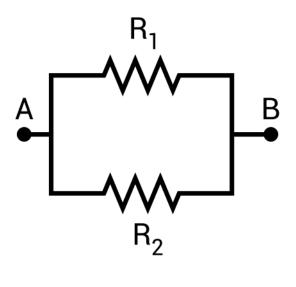
$$\frac{R_1 R_2}{R_1 + R_2}$$
