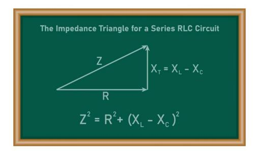
In alternating current (AC) circuits, power isn't as simple as in a DC circuit. The three types of power and the power factor help us understand how efficiently an electrical system is using its
